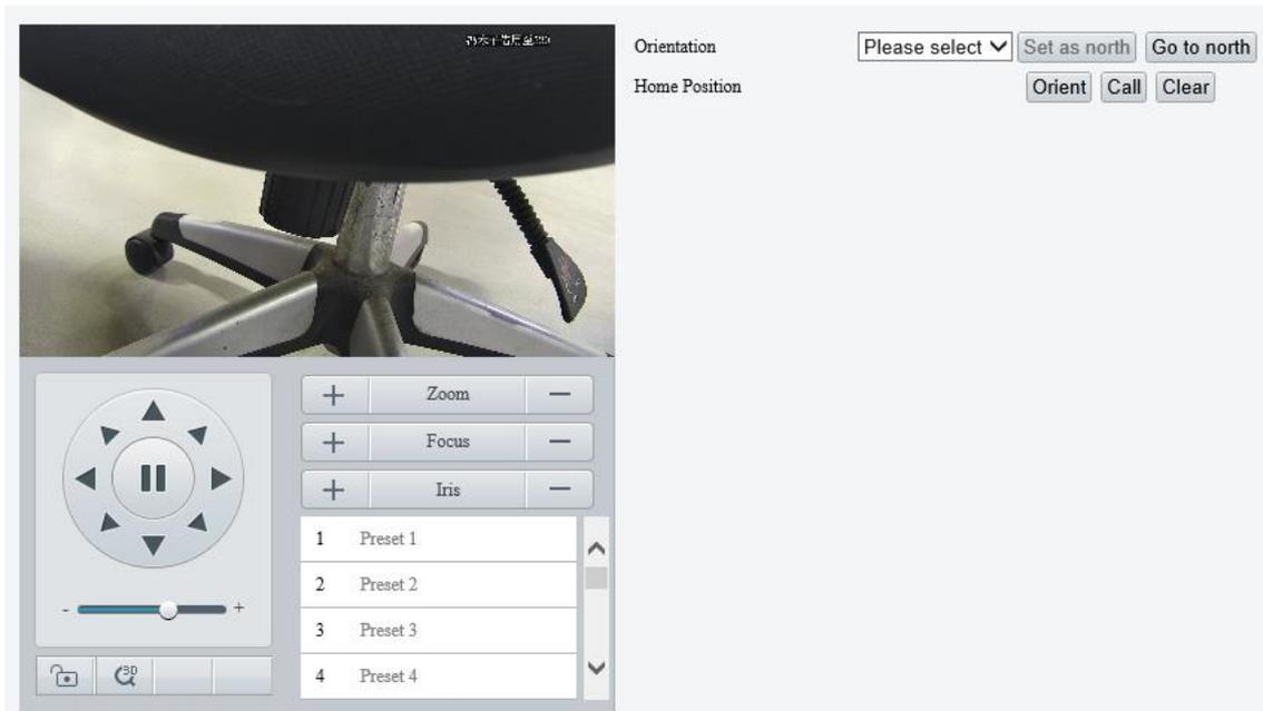
2. Select the mode to calibrate the camera to north.
