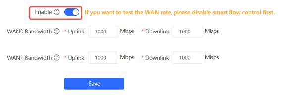
Turn on **Enable** on the **Smart QoS** tab and set the line bandwidth based on the bandwidth actually allocated by the ISP. If the device has multiple lines, you can set the bandwidth for these WAN ports separately. For details on the multi-line configuration, see Section <u>4.2</u> Port Settings.
