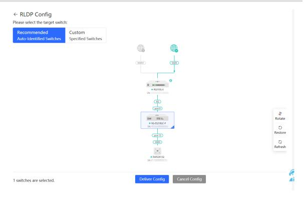
(3) After the configuration is delivered, if you want to modify the effective range of the RLDP function, click Configure to select desired switches in the topology again. Turn off RLDP to disable RLDP on all the switches with one click.
