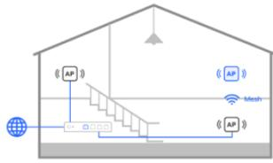
When AP Mesh is enabled, Devices that support the AP Mesh function can form a network either wirelessly or through a wired connection. The system will automatically optimize mesh links by considering factors such as signal strength, wireless mode, number of antenna streams, channel width, and signal loss across mesh hops to choose the optimal uplink.
