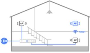
When AP Mesh is enabled, Devices that support the AP Mesh function can form a network either wirelessly or through a wired connection. The system will automatically optimize mesh links by considering factors such as signal strength, wireless mode, number of antenna streams, channel width, and signal loss across mesh hops to choose the optimal uplink.
