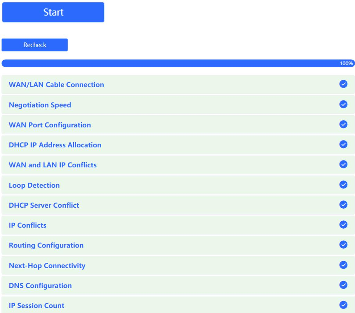
The interface displays a 'Start' button in blue. Below it is a 'Recheck' button in blue. A progress bar is shown at 100%. Below the progress bar is a list of 13 diagnostic items, each with a checkmark icon on the right:
