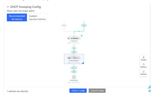
(3) After the configuration is delivered, if you want to modify the effective range of the DHCP Snooping function, click **Configure** to select desired switches in the topology again. Turn off **DHCP Snooping** to disable DHCP Snooping on all switches with one click.
